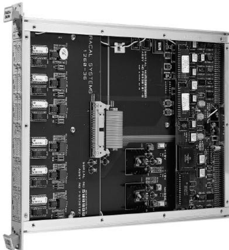
Figure 1-1, 1260-36 F.E.T. Multiplexer/Scanner Module
